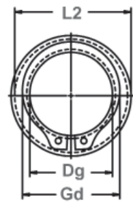
Clearance Diameter & Gaging Diameter Released in Groove.
