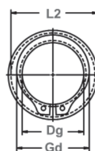
Clearance Diameter & Gaging Diameter Released in Groove.
