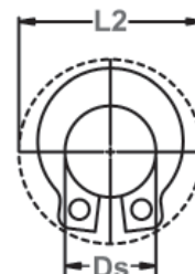
Clearance Diameter Expanded Over Shaft
