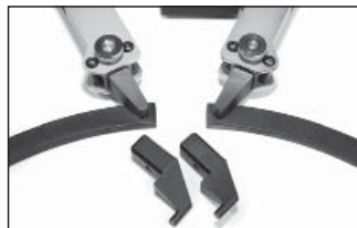
Interchangeable paired tips to cover different diameter ranges.
