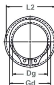
Clearance Diameter & Gaging Diameter Released in Groove.
